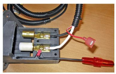
2) Position fuse lead wire into slotted area as shown. Make sure the Phillips head screw is completely tight!
